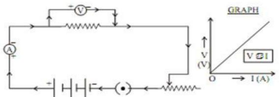
Ohm's Law  $\rightarrow$  He stated that the electric current flowing through a conductor is directly proportional to the potential difference across its ends, under standard temperature and pressur conditions.
