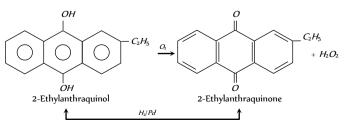
The  $H_2O_2$  formed (about 1%) is extracted with water and concentrated.
