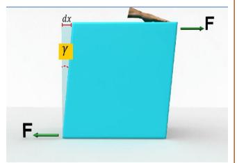
The SI unit of shear modulus is  $\ensuremath{N/m^2}$
