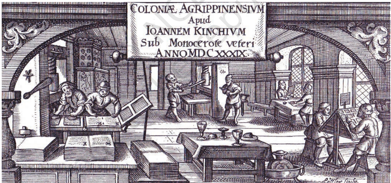
Fig. 8 – A printer’s workshop, sixteenth century. This picture depicts what a printer’s shop looked like in the sixteenth century. All the activities are going on under one roof. In the foreground on the right, compositors are at work, while on the left galleys are being prepared and ink is being applied on the metal types; in the background, the printers are turning the screws of the press, and near them proofreaders are at work. Right in front is the final product – the double-page printed sheets, stacked in neat piles, waiting to be bound.
