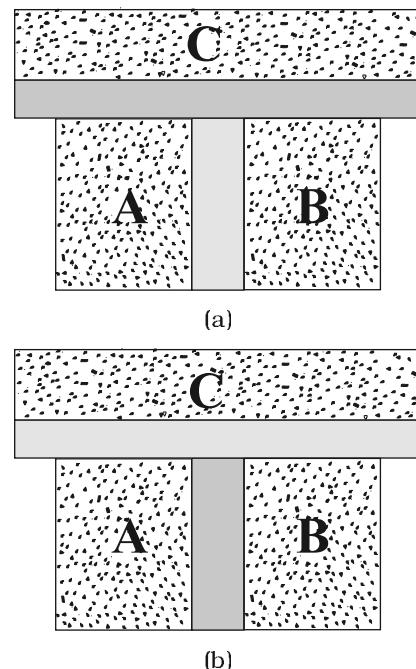
**Fig. 12.2** (a) Systems *A* and *B* are separated by an adiabatic wall, while each is in contact with a third system *C* via a conducting wall. (b) The adiabatic wall between *A* and *B* is replaced by a conducting wall, while *C* is insulated from *A* and *B* by an adiabatic wall.
