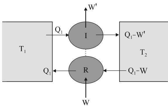
**Fig. 12.12** An irreversible engine ( $I$ ) coupled to a reversible refrigerator ( $R$ ). If  $W' > W$ , this would amount to extraction of heat  $W' - W$  from the sink and its full conversion to work, in contradiction with the Second Law of Thermodynamics.
