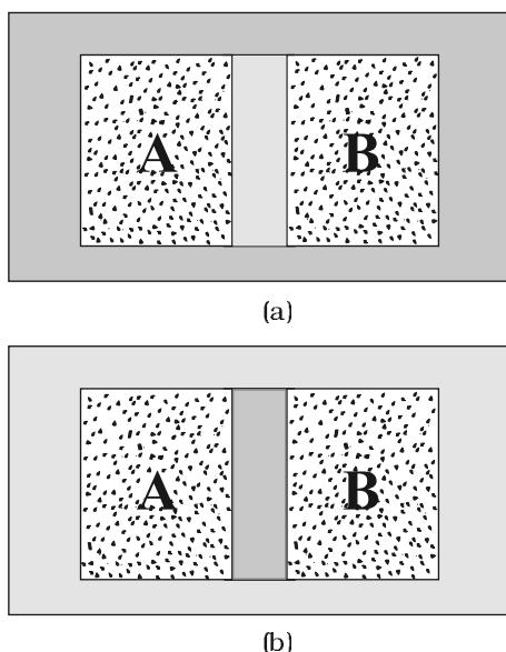
**Fig. 12.1** (a) Systems *A* and *B* (two gases) separated by an adiabatic wall – an insulating wall that does not allow flow of heat. (b) The same systems *A* and *B* separated by a diathermic wall – a conducting wall that allows heat to flow from one to another. In this case, thermal equilibrium is attained in due course.
