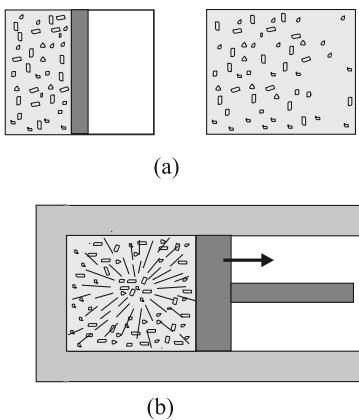
**Fig. 12.6** (a) The partition in the box is suddenly removed leading to free expansion of the gas. (b) A mixture of gases undergoing an explosive chemical reaction. In both situations, the gas is not in equilibrium and cannot be described by state variables.
