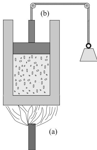
**Fig. 12.4** Heat and work are two distinct modes of energy transfer to a system that results in change in its internal energy. (a) Heat is energy transfer due to temperature difference between the system and the surroundings. (b) Work is energy transfer brought about by means (e.g. moving the piston by raising or lowering some weight connected to it) that do not involve such a temperature difference.
