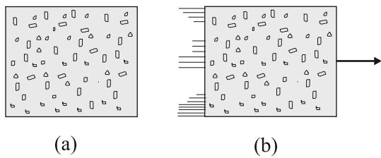
**Fig. 12.3** (a) Internal energy  $U$  of a gas is the sum of the kinetic and potential energies of its molecules when the box is at rest. Kinetic energy due to various types of motion (translational, rotational, vibrational) is to be included in  $U$ . (b) If the same box is moving as a whole with some velocity, the kinetic energy of the box is not to be included in  $U$ .
