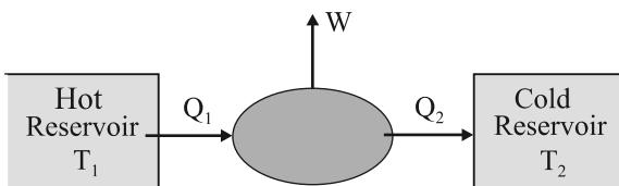
**Fig. 12.9** Schematic representation of a heat engine. The engine takes heat  $Q_1$  from a hot reservoir at temperature  $T_1$ , releases heat  $Q_2$  to a cold reservoir at temperature  $T_2$  and delivers work  $W$  to the surroundings.
