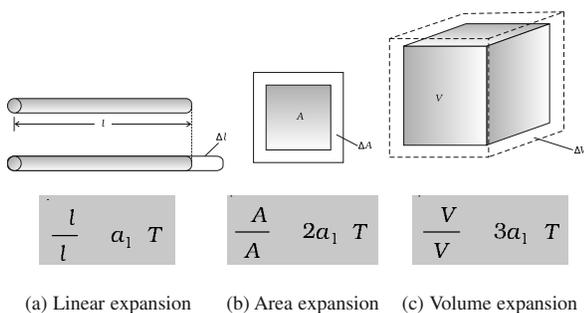
Fig. 11.5 Thermal Expansion.
