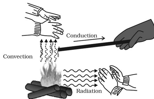
**Fig. 11.13** Heating by conduction, convection and radiation.
