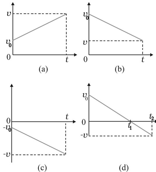
**Fig. 3.10** Velocity-time graph for motions with constant acceleration. (a) Motion in positive direction with positive acceleration, (b) Motion in positive direction with negative acceleration, (c) Motion in negative direction with negative acceleration, (d) Motion of an object with negative acceleration that changes direction at time  $t_1$ . Between times 0 to  $t_1$ , its moves in positive  $x$ -direction and between  $t_1$  and  $t_2$  it moves in the opposite direction.
