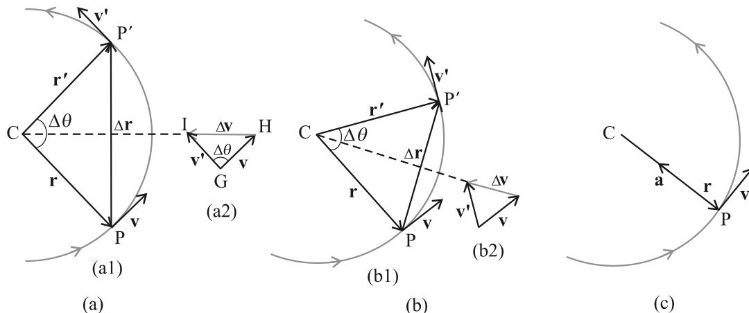
**Fig. 4.19** Velocity and acceleration of an object in uniform circular motion. The time interval  $\Delta t$  decreases from (a) to (c) where it is zero. The acceleration is directed, at each point of the path, towards the centre of the circle.
