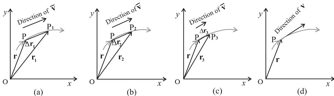
**Fig. 4.13** As the time interval  $\Delta t$  approaches zero, the average velocity approaches the velocity  $\mathbf{v}$ . The direction of  $\bar{\mathbf{v}}$  is parallel to the line tangent to the path.
