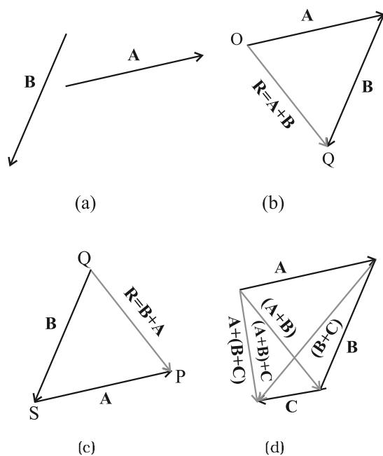
**Fig. 4.4** (a) Vectors  $\mathbf{A}$  and  $\mathbf{B}$ . (b) Vectors  $\mathbf{A}$  and  $\mathbf{B}$  added graphically. (c) Vectors  $\mathbf{B}$  and  $\mathbf{A}$  added graphically. (d) Illustrating the associative law of vector addition.
