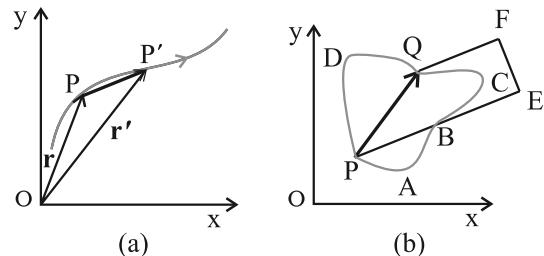
**Fig. 4.1** (a) Position and displacement vectors.
