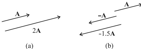
**Fig. 4.3** (a) Vector  $\mathbf{A}$  and the resultant vector after multiplying  $\mathbf{A}$  by a positive number 2. (b) Vector  $\mathbf{A}$  and resultant vectors after multiplying it by a negative number  $-1$  and  $-1.5$ .
