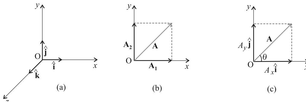
Fig. 4.9 (a) Unit vectors  $\hat{i}$ ,  $\hat{j}$  and  $\hat{k}$  lie along the  $x$ -,  $y$ -, and  $z$ -axes. (b) A vector  $\mathbf{A}$  is resolved into its components  $\mathbf{A}_1$  and  $\mathbf{A}_2$  along  $x$ - and  $y$ -axes. (c)  $\mathbf{A}_1$  and  $\mathbf{A}_2$  expressed in terms of  $\hat{i}$  and  $\hat{j}$ .
