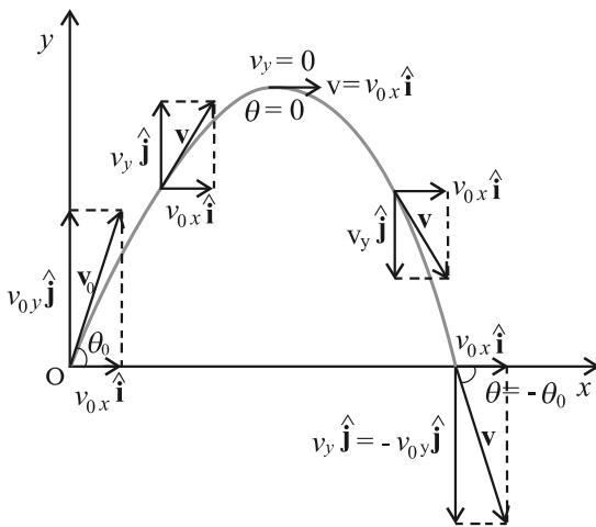
**Fig. 4.18** The path of a projectile is a parabola.
