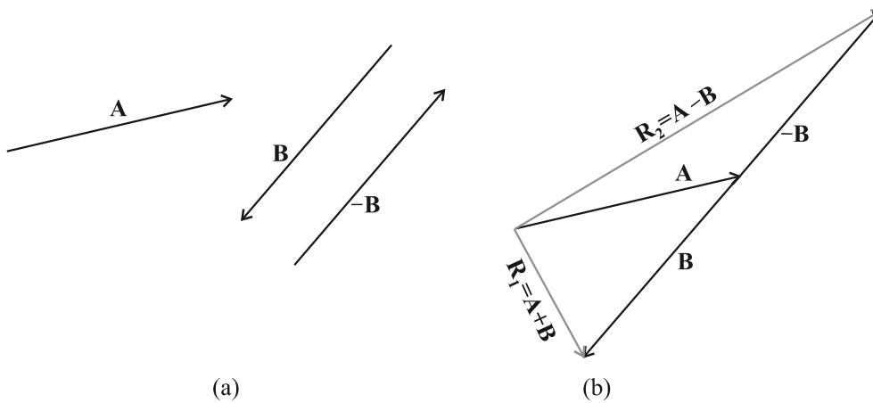
Fig. 4.5 (a) Two vectors  $\mathbf{A}$  and  $\mathbf{B}$ ,  $-\mathbf{B}$  is also shown. (b) Subtracting vector  $\mathbf{B}$  from vector  $\mathbf{A}$  – the result is  $\mathbf{R}_2$ . For comparison, addition of vectors  $\mathbf{A}$  and  $\mathbf{B}$ , i.e.  $\mathbf{R}_1$  is also shown.
