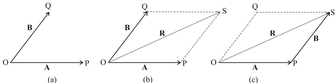
**Fig. 4.6** (a) Two vectors **A** and **B** with their tails brought to a common origin. (b) The sum **A + B** obtained using the parallelogram method. (c) The parallelogram method of vector addition is equivalent to the triangle method.
