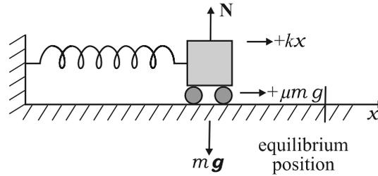
Fig. 6.9 The forces acting on the car.
