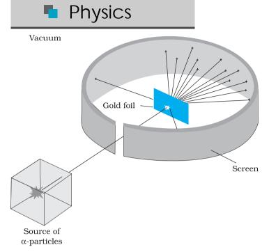
**FIGURE 12.1** Geiger-Marsden scattering experiment. The entire apparatus is placed in a vacuum chamber (not shown in this figure).
