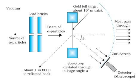
FIGURE 12.2 Schematic arrangement of the Geiger-Marsden experiment.
