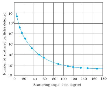
**FIGURE 12.3** The dots are  $\alpha$ -particle scattering data for a thin gold foil obtained by Geiger and Marsden using the experiment shown in Figs. 12.1 and 12.2. The solid curve is the theoretical prediction based on the assumption that atom has a small, dense, positively charged nucleus.
