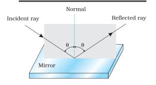
**FIGURE 9.1** The incident ray, reflected ray and the normal to the reflecting surface lie in the same plane.
