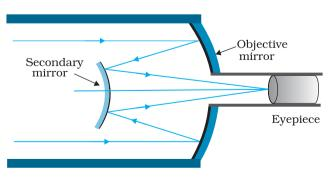
**FIGURE 9.33** Schematic diagram of a reflecting telescope (Cassegrain).
