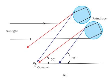
FIGURE 9.27 Rainbow: (a) The sun rays incident on a water drop get refracted twice and reflected internally by a drop; (b) Enlarge view of internal reflection and refraction of a ray of light inside a drop form primary rainbow; and (c) secondary rainbow is formed by rays undergoing internal reflection twice inside the drop.
