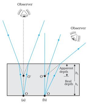
**FIGURE 9.10** Apparent depth for (a) normal, and (b) oblique viewing.
