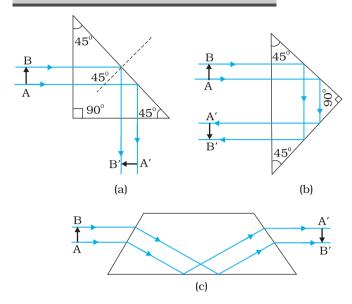
**FIGURE 9.15** Prisms designed to bend rays by 90° and 180° or to invert image without changing its size make use of total internal reflection.
