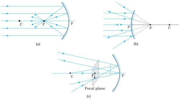
FIGURE 9.3 Focus of a concave and convex mirror.
