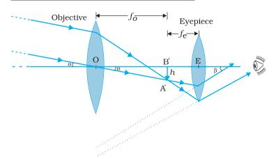
**FIGURE 9.32** A refracting telescope.
