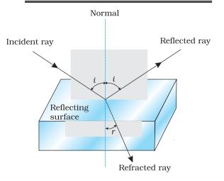
**FIGURE 9.8** Refraction and reflection of light.
