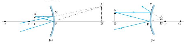
**FIGURE 9.6** Image formation by (a) a concave mirror with object between P and F, and (b) a convex mirror.
