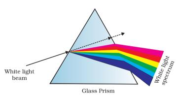
**FIGURE 9.25** Dispersion of sunlight or white light on passing through a glass prism. The relative deviation of different colours shown is highly exaggerated.
