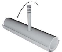
Fig. 8.4 Directions of movement allowed by a hinge like joint
