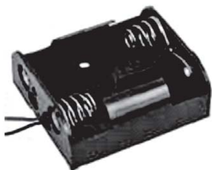
Fig. 14.5 Holder for battery of two cells
