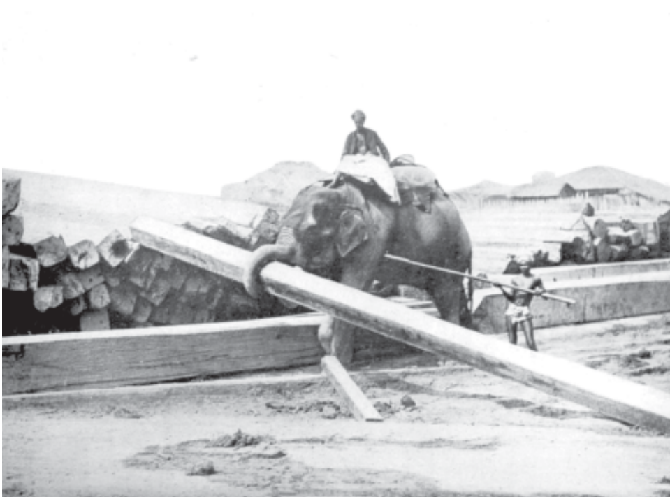
Fig.5 – Elephants piling squares of timber at a timber yard in Rangoon. In the colonial period elephants were frequently used to lift heavy timber both in the forests and at the timber yards.
