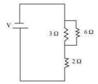
Here, 6  $\Omega$  and 3  $\Omega$  resistors are connected in parallel.
