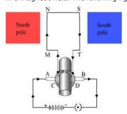
When a current is allowed to flow through the coil MNST by closing the switch, the coil starts rotating anti-clockwise. This happens because a downward force acts on length MN
