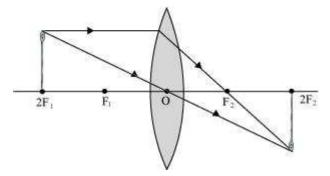
It is given that the image of the needle is formed at a distance of 50 cm from the convex lens. Hence, the needle is placed in front of the lens at a distance of 50 cm.
