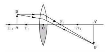
An object 5 cm in length is held 25 cm away from a converging lens of focal length 10 cm. Draw the ray diagram and find the position, size and the nature of the image formed.
