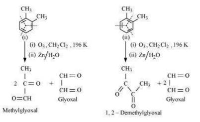
All three products, i.e., methyl glyoxal, 1, 2-demethylglyoxal, and glyoxal are obtained from two Kekule structures. Since all three products cannot be obtained from any one of the two structures, this proves that *o*-xylene is a resonance hybrid of two Kekule structures (I and II).
