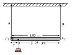
Taking torque about the point of suspension, we have:
