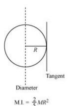
According to the theorem of parallel axes, the moment of inertia of a body about any axis is equal to the sum of the moment of inertia of the body about a parallel axis passing through its centre of mass and the product of its mass and the square of the distance between the two parallel axes.
