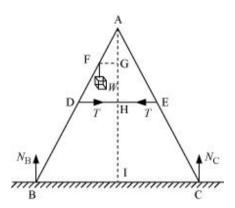
$N_B$  = Force exerted on the ladder by the floor point B
