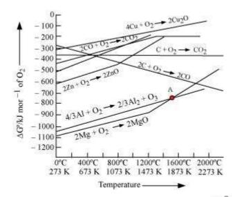
The above figure is a plot of Gibbs energy  $(\Delta G^{\circ})$ vs. T for formation of some oxides.
