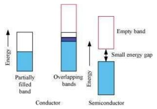
On the other hand, the valence band of a semiconductor is filled and there is a small gap between the valence band and the next higher conduction band. Therefore, some electrons can jump from the valence band to the conduction band and conduct electricity.
