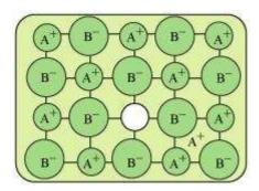
(iii) Interstitials: Interstitial defect is shown by non-ionic solids. This type of defect is created when some constituent particles (atoms or molecules) occupy an interstitial site of the crystal. The density of a substance increases because of this defect.
