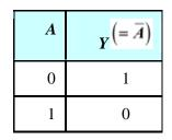
This circuit functions as a NOT gate. The symbol for this logic circuit is shown as:
