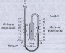
Fig. 4.3 A type of maximum and minimum thermometer.
