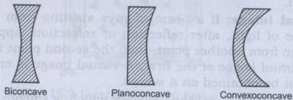
Fig. 15.5 Different types of concave lenses.
