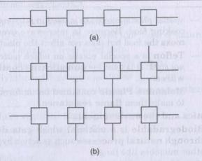
Fig. 3.1 (a) Linear (b) Cross-linked arrangement.
