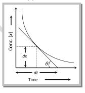
Where, d[A], d[B] and dt being infinitesimally small changes in the concentration of A and B, that of time respectively. Instantaneous rate of reaction at any instant of time is obtained by finding the slope of the tangent to the curve (which is obtained by plotting concentration of any suitable reactant or product versus time) at the point corresponding to that instant of time. Rate of reaction =  $\tan \theta = \frac{dx}{dt}$
