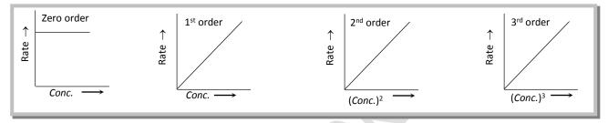
(4) **Van't Haff differential Method:** The rate of reaction varies as the n<sup>th</sup> power of the concentration where '*n*' is the order of the reaction. Thus for two different initial concentrations  $C_1$  and  $C_2$  equation,
