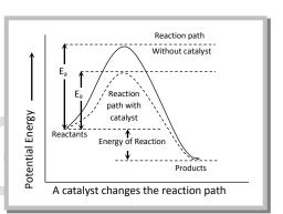
are able to cross over the energy barrier and thus the rate of reaction increases. Fig. shows how the activation energy is lowered in presence of a catalyst.
