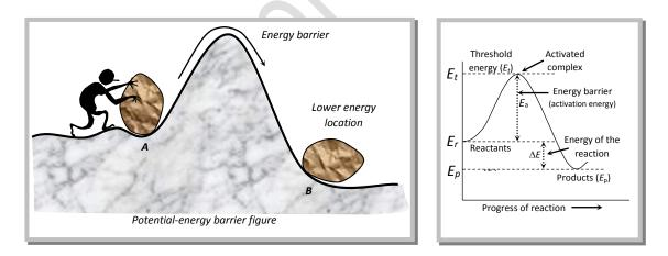
Note: The activation energy is found to increase with the lowering of temperature i.e., at lower temperatures the activation energy tends to increase.
