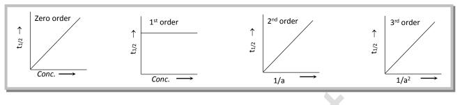
(3) Graphical method: A graphical method based on the respective rate laws, can also be used.
