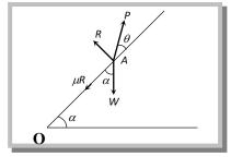
(2) Least force required to pull a body down an inclined plane: Let a body of weight W be at the
