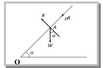
Thus, if a body be on the point of sliding down an inclined plane under its own weight, the inclination of the plane is equal to the angle of the friction.
