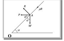
Note: If  $\alpha = \lambda$ , then the body is in limiting equilibrium and is just on the point of moving downwards.
