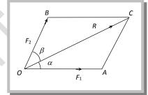
$$F_1 = \frac{OC.\sin\beta}{\sin(\alpha + \beta)} = \frac{R\sin\beta}{\sin(\alpha + \beta)} \text{ and } F_2 = \frac{OC.\sin\alpha}{\sin(\alpha + \beta)} = \frac{R.\sin\alpha}{\sin(\alpha + \beta)}$$
