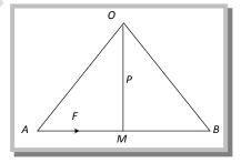
(1) **Sign of the moment:** The moment of a force about a point measures the tendency of the force to cause rotation about that point. The tendency of the force  $F_1$  is to turn the lamina in the
