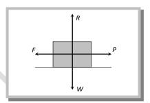
(1) **Friction is a self-adjusting force:** Let a horizontal force P pull a heavy body of weight W resting on a smooth horizontal table. It will be noticed that up to a certain value of P, the body does not move. The reaction R of the table and the weight W of the body do not have any effect on the horizontal pull as they are vertical. It is the force of friction F, acting in the horizontal direction, which balances P and prevents the body from moving.
