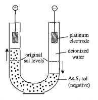
Electrophoresis is used to determine the charge on colloidal particles, if particle move towards negative electrode, the charge on the particle is positive and viceversa.
