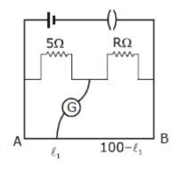
Option A 100Ω Option B 15Ω Option C 20Ω Option D 25Ω **Correct Option B** Solution: At balance point  $\frac{5}{R}=\frac{\ell_1}{100-\ell_1}$ After shunting  $\frac{5}{R\,/\,2} = \frac{1.6\ell_1}{100 - 1.6\ell_1}$ On solving  $\Rightarrow$  R = 15  $\Omega$
