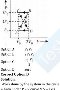
= Area under P – V curve & V – axisFor clockwise work done is positiveFor anticlockwise work done is negative
