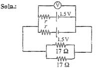
Let the internal resistance of each cell is 'r' on equivalent simplified circuit can be drawn
