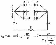
In case of mixed grouping of cells, current in the circuit will be maximum, when
