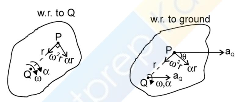
$\theta$ ,  $\omega$ ,  $\alpha$  are same about every point of the body (or any other point outside which is rigidly attached to the body).
