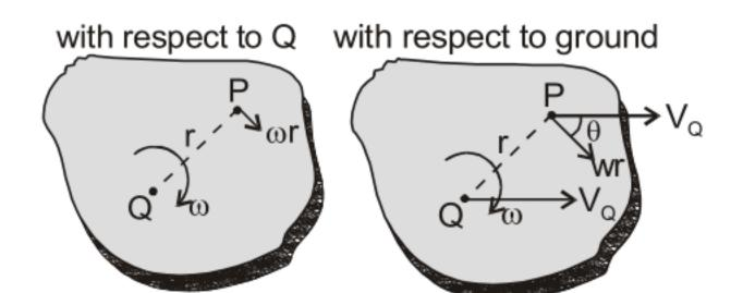
$$V_{P} = \sqrt{V_{Q}^{2} + (\omega r)^{2} + 2 V_{Q} \omega r \cos \theta}$$
