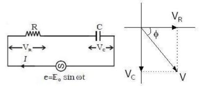
Suppose in phasor diagram current is taken along positive x-direction. Then  $v_R$  is along positive x-direction but  $V_C$  is along negative y-direction as current leads the potential by phase  $90^{\circ}$  so we can write
