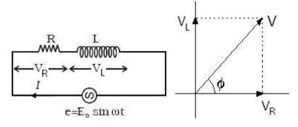
Suppose in phasor diagram, current is taken along positive direction. The V<sub>R</sub> is also along positive x-direction as there is no phase difference between  $i_R$  and  $V_R$ . While V<sub>L</sub> will be along y direction as we know that current lags behind the voltage by 90<sup>0</sup> So we can write
