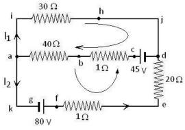
Junction or Branch point: The point in network at which more than two conductors meet is called a junction or a branch point . Point a and d shown in figure are junction point .
