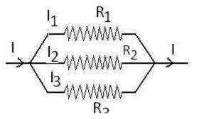
Two or more resistors are said to be connected in parallel if one end of all the resistors is joined together and similarly the other ends are joined together as shown in figure.
