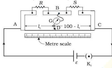
It consists of a wire of length 1m and of uniform cross sectional area stretched taut and clamped between two thick metallic strips bent at right angles, as shown.
