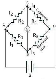
The circuit shown in figure which is called the Wheatstone bridge. The bridge has four resistors  $R_1$ ,  $R_2$ ,  $R_3$  and  $R_4$ . Across one pair of diagonally opposite points (A and C in the figure) a source is connected. This (i.e., AC) is called the battery arm.
