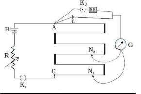
For this the cell (emf  $\varepsilon$ ) whose internal resistance (*r*) is to be determined is connected across a resistance box through a key K<sub>2</sub>, as shown in the figure. With key K<sub>2</sub> open, balance is obtained at length l<sub>1</sub> (AN<sub>1</sub>). Then,
