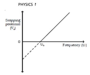
From this graph, it is found that at a frequency  $v_0$ , the value of the stopping potential is zero. This frequency is known as the threshold frequency for the photo metal used. The photoelectric effect occurs above this frequency and ceases below it.
