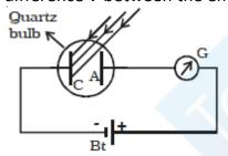
The amount of current passing through the ammeter gives an idea of the number of photoelectrons. At some value of positive potential difference, when all the emitted electrons are collected, increasing the potential difference further has no effect on the current.
