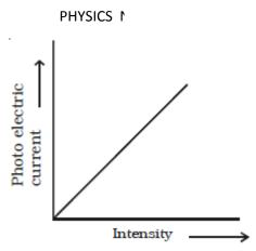
Since the photoelectric current is directly proportional to the number of photoelectrons emitted per second, it implies that the number of photoelectrons emitted per second is proportional to the intensity of incident radiation.
