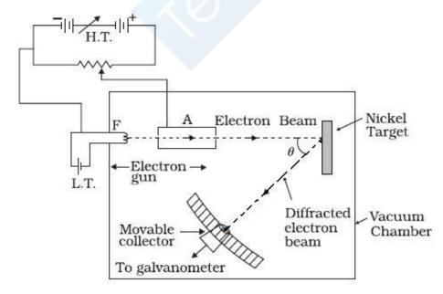
It consists of an electron gun wnich comprises of a tungsten filament F, coated with barium oxide and heated by a low voltage power supply (L.T. or battery).
