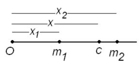
distance of  $x_1$  and  $x_2$  respectively from the origin (O). The centre of mass of this system is that point whose distance from origin O is given by  $x = \frac{m_1 x_1 + m_2 x_2}{m_1 x_1 + m_2 x_2}$
