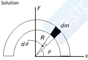
From the symmetry of the body we see at once that the centre of mass of the body must lie along y-axis. So  $X_{CM} = 0$ .
