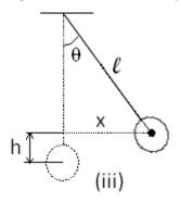
Then potential energy at the new position U = mgl(1-cos $\theta$ ) Kinetic energy at this instant K = (1/2) mv<sup>2</sup> Total mechanical energy at this instant E = U + K E = mgl(1-cos $\theta$ ) + (1/2) mv<sup>2</sup> We know, in simple harmonic motion E = constant  $\frac{dE}{dt} = 0$
