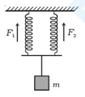
mass m having non-uniform density distribution is suspended so that spring undergoes equal extension
