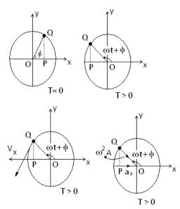
In figure shown Q is a point moving on a circle of radius A with constant angular speed  $\omega$  (in rad/sec). P is the perpendicular projection of Q on the horizontal diameter, along the x-axis.
