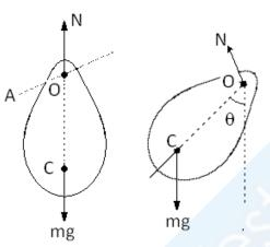
As shown in figure is a physical pendulum. A rigid body is suspended through a hole at O. When the centre of mass C is vertically below O at a distance of 'l', the body may remain at rest.
