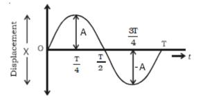
Mathematical equation is the function of time  $x(t) = Asin(\omega t + \varphi) ----eq(1)$ Here X(t) represents displacement at time t A = Amplitude ( $\omega t + \varphi$ ) = Phase  $\varphi$  = Initial phase (epoch) for a given graph  $\varphi$ = 0. If oscillation have started from negative x end (M) then initial phase is  $-\pi/2$ If oscillation stated from positive end (N) then initial phase is  $\pi/2$  $\omega$  = angular frequency
