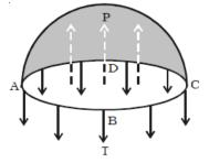
Imagine the drop to be divided into two equal halves. Considering the equilibrium of the upper hemisphere of the drop, the upward force on the plane face ABCD due to excess pressure *P* is  $P \pi r^2$
