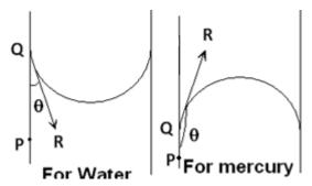
When the free surface of a liquid comes in contact with a solid, it becomes curved at the point of contact. The angle between the tangent to the liquid surface at the point of contact of the liquid with the solid and the solid surface inside the liquid is called angle of contact. In Fig., QR is the tangent drawn at the point of contact Q. The angle PQR is called the angle of contact. When a liquid has
