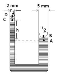
each surface exceeds that on the convex side by 2T/r, where T is surface tension and r is the radius of the limb concerned Now  $r_1 = 2.5 \text{ mm} = 2.5 \times 10^{-3} \text{ m}$  and  $r_2 = 1 \text{ mm} = 10^{-3} \text{ m}$ Hence
