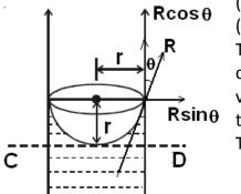
(i) Horizontal component *R* sin  $\theta$  acting radially outwards (ii) Vertical component *R* cos  $\theta$  acting upwards. The horizontal component acting all along the
