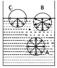
The surface tension of liquid arises out of the attraction of its molecules. Molecules of fluid (liquid and gas) attract one another with a force. If any other molecule is within the sphere of influence of first molecule it will experience a force of attraction
