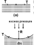
has no component perpendicular to the horizontal surface. As a result, there is no pressure difference between the liquid side and the vapour side.
