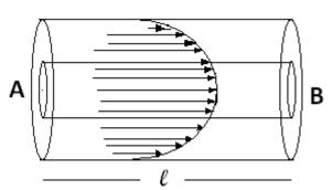
To maintain such flow, the force balancing the viscous force obtained by producing the pressure difference(P) across the ends of the tube. Derive the equation of velocity of a layer situated at distance 'x' from the axis of the tube
