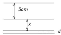
Consider a layer of thickness dx and surface area A. Heat required to b taken out from such layer is  $dQ = Adx \rho L$
