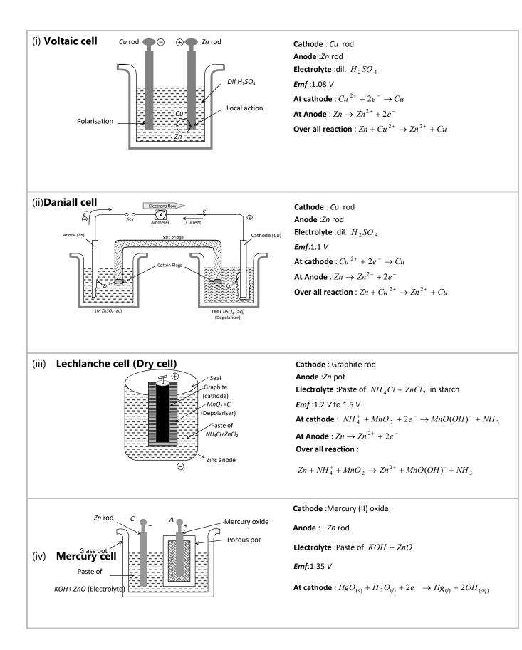
Note: In a dry cell  $ZnCl_2$  combines with  $NH_3$  produced to form the complex  $[Zn(NH_3)_2 Cl_2]$ , otherwise the pressure developed due to  $NH_3$  would crack the seal of the cell.
