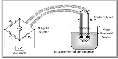
The second difficulty can be solved by using a specially designed vessels called **conductivity cell**.
