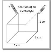
In SI units, I is expressed in m area of cross-section in  $m^2$  so that the units of conductivity are S  $m^{-1}$ .
