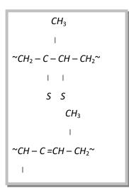
In a polymer, the chains are normally tangled up with each other. When the rubber is stretched, the chains straighten out to some extent. The chains cannot slip past each other because of the polysulphide bridges. Thus, rubber can be stretched only to a limited extent. When the tension is removed, the chains try to coil up again and the rubber resumes its original shape.
