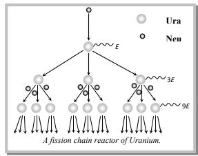
Note: Each fission yields 3 neutrons each of which can cause further fission to give 3 neutrons goes on increasing in geometric progression 1,
