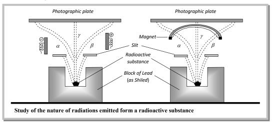
It is observed that on applying the field, the rays emitted from the radioactive substances are separated into three types, called  $\alpha$ ,  $\beta$ , and  $\gamma$ -rays. The  $\alpha$ -rays are deflected in a direction which shows that they carry positive charge; the  $\beta$ -rays are deflected in the opposite direction showing that they carry negative charge and the  $\gamma$ -rays are not deflected at all showing that they carry no charge.
