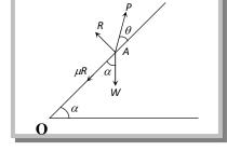
(2) **Least force required to pull a body down an inclined plane:** Let a body of weight W be at the point A,  $\alpha$  be the inclination of rough inclined plane to the horizontal and  $\lambda$  be the angle of friction. Let P be the force acting an angle  $\theta$  with the plane, required just to move the body up the plane.
