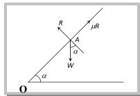
Thus, if a body be on the point of sliding down an inclined plane under its own weight, the inclination of the plane is equal to the angle of the friction.
