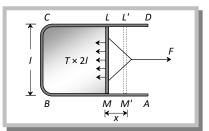
If T is the force due to surface tension per unit length, then F = T  $\times$  2I
