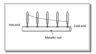
After sometime, a state is reached when the temperature of every cross-section of the rod becomes constant. In this state, no heat is absorbed by the rod. The heat that reaches any cross-section is transmitted to the next except that a small part of heat is lost to surrounding from the
