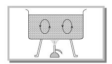
(2) Forced convection: If a fluid is forced to move to take up heat from a hot body then the convection process is called forced convection. In this case Newton's law of cooling holds good. According to which rate of loss of heat from a hot body due to moving fluid is directly proportional to the surface area of body and excess temperature of body over its surroundings
