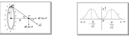
(a) **Electric field:**Consider an element carrying charge dQ. Its electric field  $dE = \frac{KdQ}{(R^2 + x^2)}$  directed as shown. Its component along the axis is  $dE \cos \theta$  and perpendicular to the axis is
