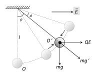
On displacing the bob from its equilibrium position 0'. It will oscillate under the effective acceleration g', where
